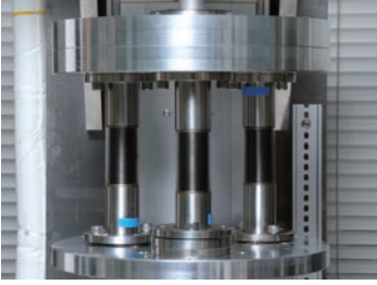
Bellows Cycle Life Testing
